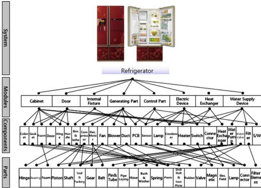
Fig. 7.6 Breakdown of a refrigeration system with multi-modules
