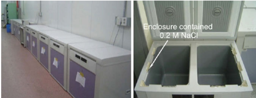
(a) Kimchi refrigerators in testing with 0.2 M NaCl water solution on evaporator
