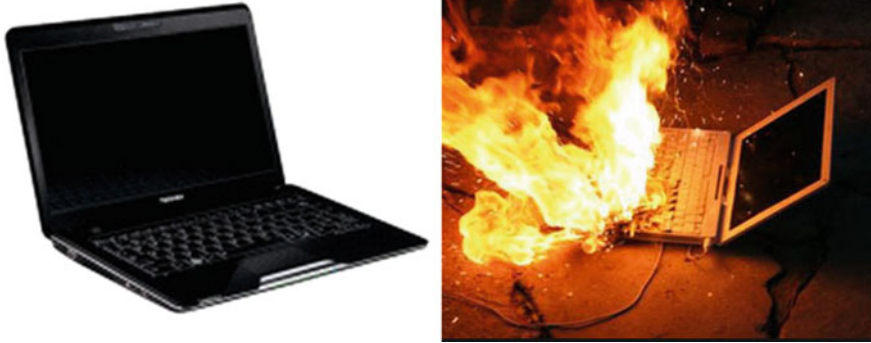
Fig. 2.10 Toshiba Satellite T130 notebook and battery overheating problem
