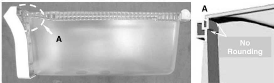
Fig. 8.93 Structure of failing drawer system in field
